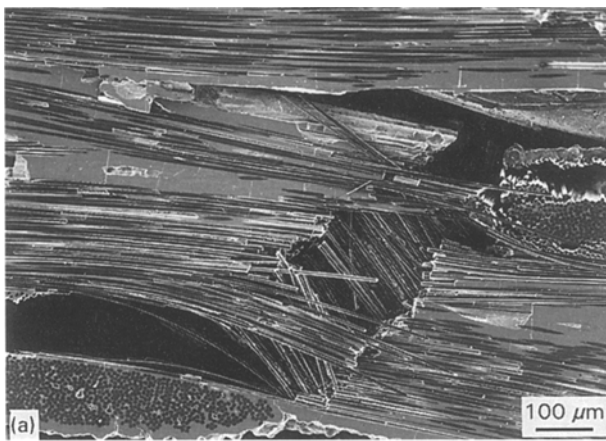
Figure 5 Optical micrograph showing compression fracture of a C/SiC composite. Note that longitudinal bundles fracture in groups of two (A) and they lie about a macroscopic shear plane across the sample, indicated by the oblique line.
